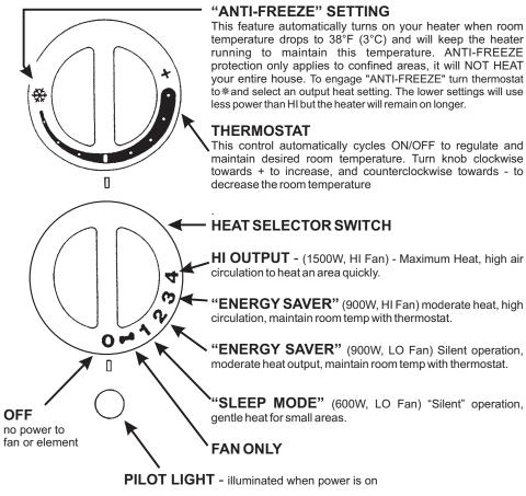
NOTE: If the pilot light is on but the heater isn't working, turn the thermostat in a clockwise direction.
